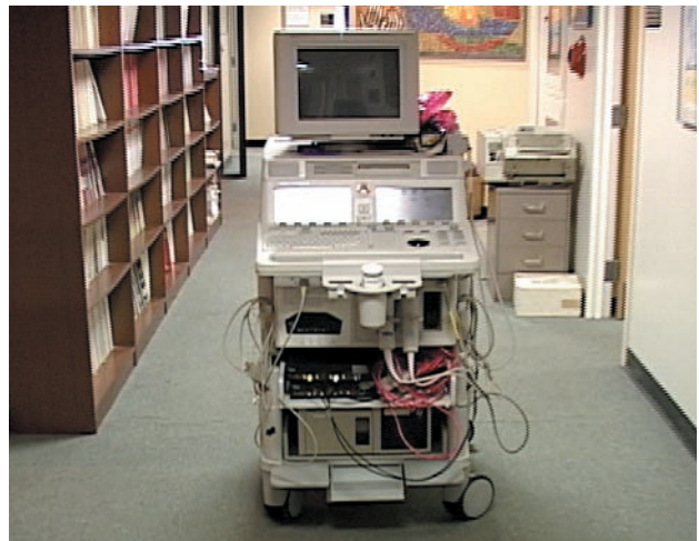
Ultrasonic equipment cart with VBrick 6200 MPEG-2 encoder
