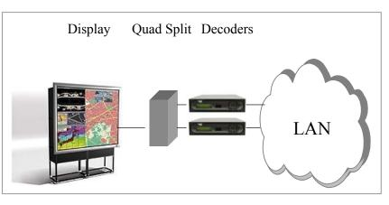
available equipment. Two VBrick decoders, for example, can decode four MPEG-2 channels and present these to a "Quad Split" device for presentation. Each VBrick channel is independently controlled over the network and each channel may continuously scan the live video feeds.
