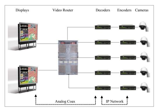
presupposes a system to control the video router (i.e. the video matrix switch).
