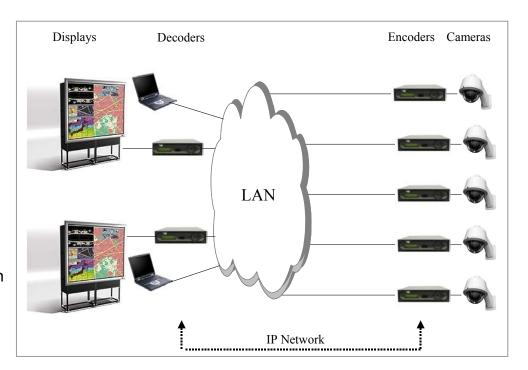
the decoder and causes it to "scan" any number of video streams, displaying each video on the display for a specified period. In addition, those same videos are
