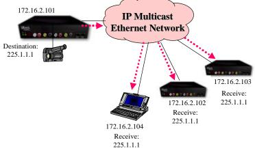
Introduction to Multicasting Copyright VBrick Systems, Inc. streams or to engage other data traffic. Routers periodically ask the members of a multicast group if they are still active, and will stop sending multicast traffic to a client when either of two things occur:
