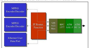
concentrate IP traffic across the ATM network. The VBrick internal routing function automatically knows which ATM interface is most appropriate to use based upon routing knowledge leaned through the RIP processing. VBrick can seamlessly convert between Ethernet and ATM IP layers, and automatically extract video and management IP packets. The local Ethernet interface port may be used as an data access port, such that IP data presented to it is automatically routed to a particular ATM PVC.
