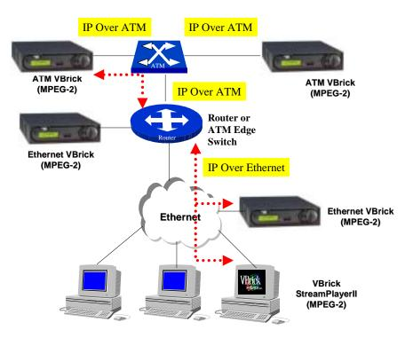
Service providers, cable operators, and content aggregators benefit from IP over ATM because, at some point along the delivery chain, the network infrastructure will presuppose IP. Some Digital Subscriber Line Access
