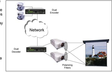
Both the encoders and decoders support composite and S-Video, and both support CD-quality stereo audio.
